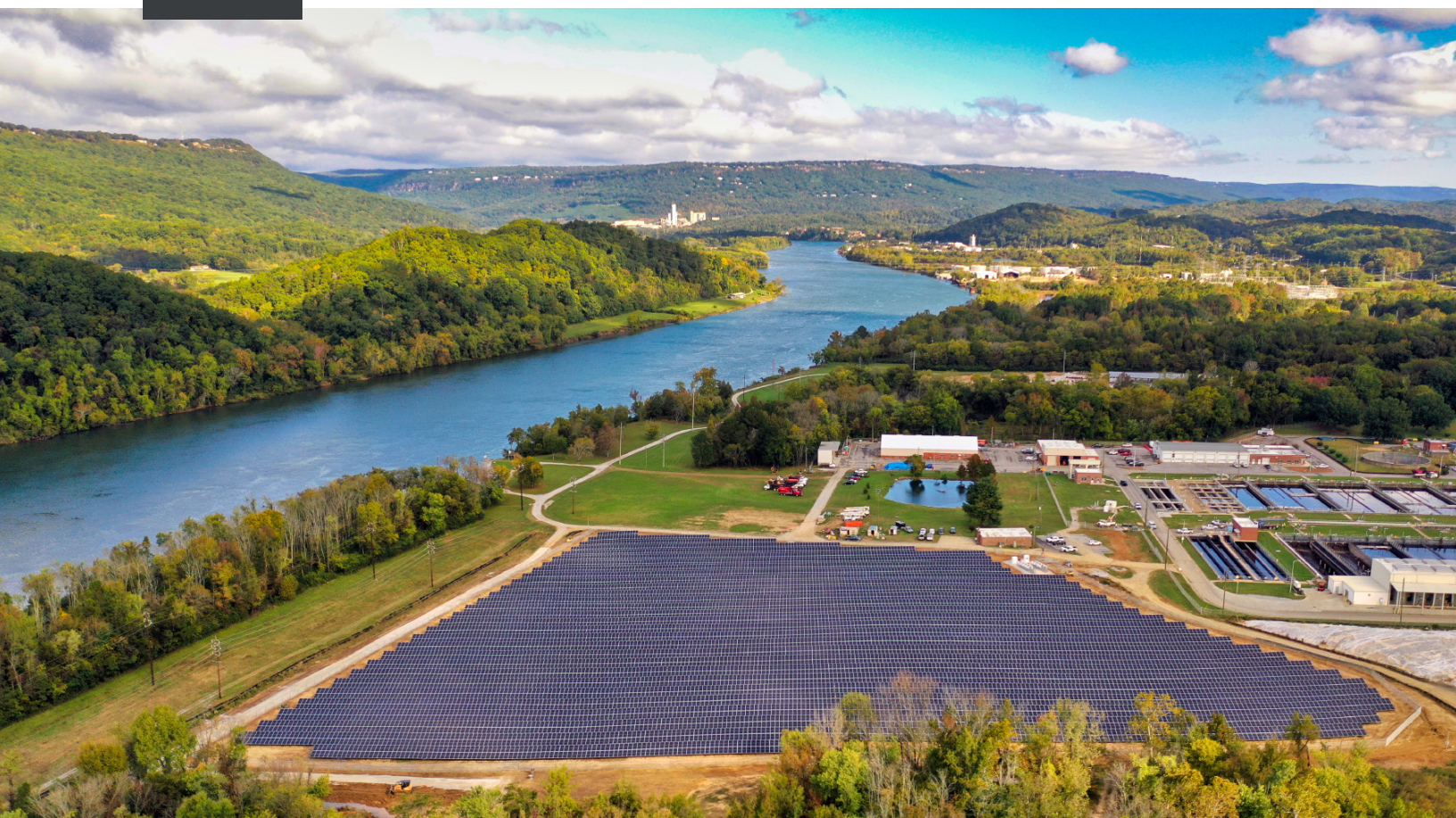
4 megawatt solar array at the Moccasin Bend Environmental Campus (regional wastewater treatment plant).
